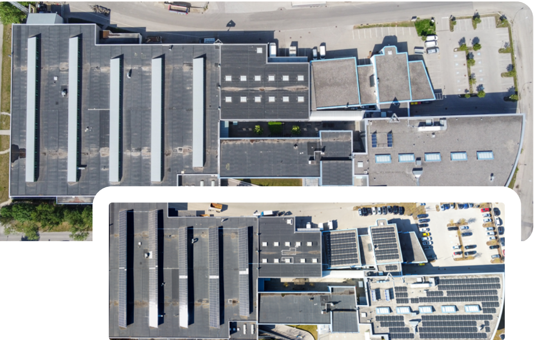
Figure 3: Top view of the site with its four industrial buildings before and after the installation of the PV system. (Source: GW St. Pölten)
